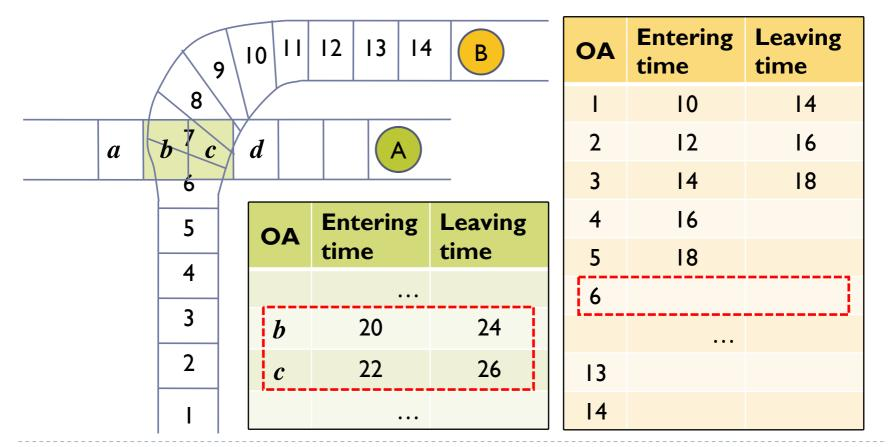
Travel Time Estimation and Deadlock-free Routing of an AGV system
