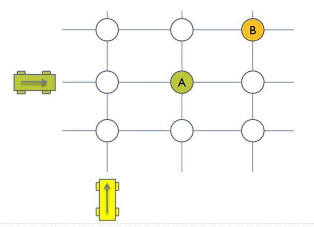
To avoid collision, only one AGV is allowed to occupy a zone at a time
