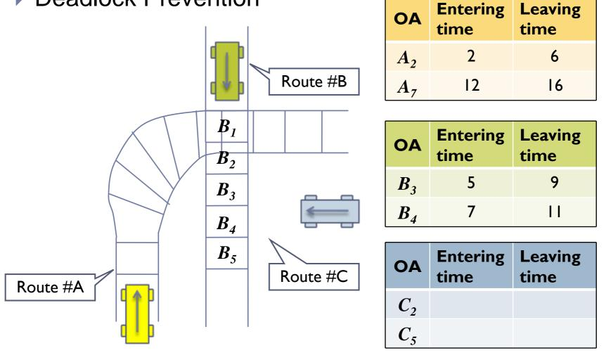
Travel Time Estimation and Deadlock-free Routing of an AGV system
